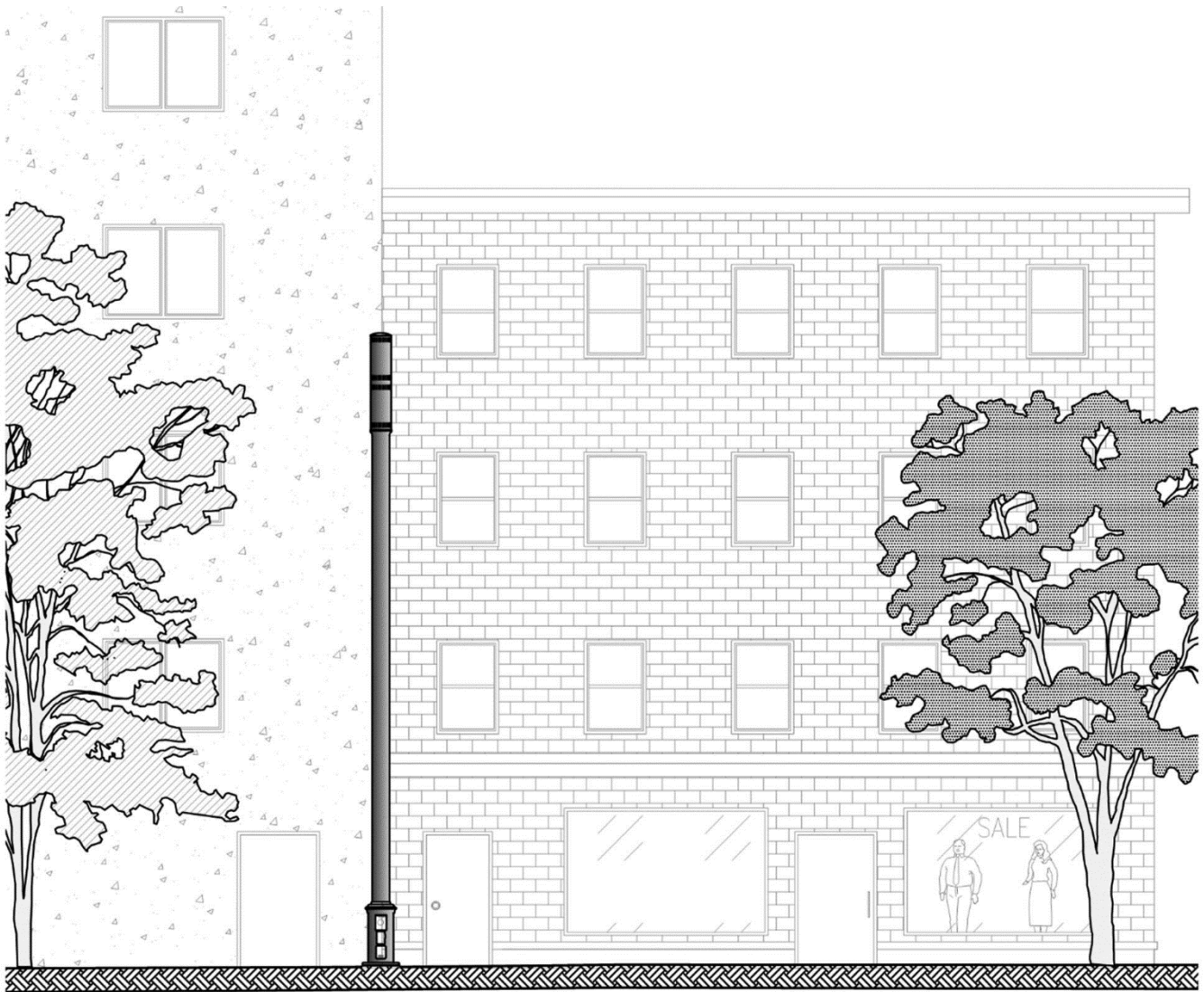
Figure 5-9: Small Cell in Commercial Area
